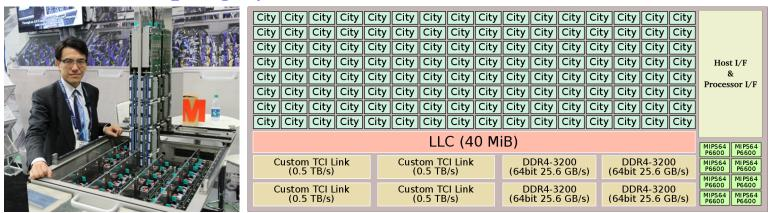
ThruChip Interface (TCI): Interchip communication through magnetic coupling
