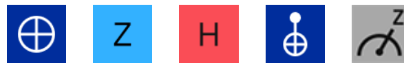
Fig. 9: Symbols for Pauli X (NOT), Pauli Z, Hadamard (H), conditional not (CNOT) and measurement gates used in IBM Q Composer.
