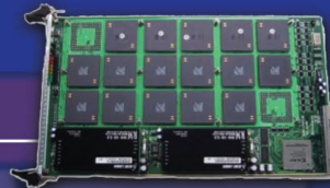
A WINE-2 system board
