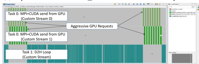
(b) Impact of manual MPI+GPU send task with concurrent D2H operations.
