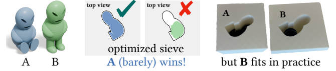
Fig. 14. It can happen that we determine that \mathcal{A} has won, but \mathcal{B} is blocked by such a tiny amount that, when printed, it still passes the sieve. This can sometimes be overcome by increasing the rasterization resolution or (similarly) scaling the meshes.
