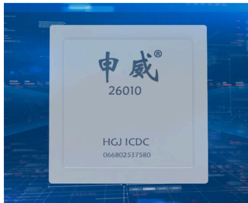
Figure 3: Image of SW26010 many-core (260 core) processor that makes up the node.
