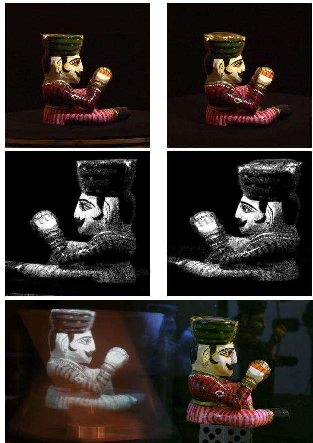
Figure 9: (Top row) Two images from an object light field captured using a turntable. (Middle row) Resampled projector frames optimized for the same two viewer heights. Both frames compensate for the horizontal divergence of projector rays and vertical stretching at oblique viewing angles. The images appear mirror-reversed (and for most views, rotated) prior to projection. (Bottom row) A single photograph of the original object sitting to the right of its virtual version shown on the 3D display.
