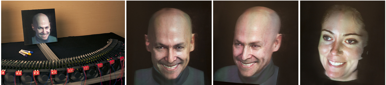
Figure 1: Our projector array (left) generates autostereoscopic views of a virtual character (middle) and 4D facial performance capture (right)
