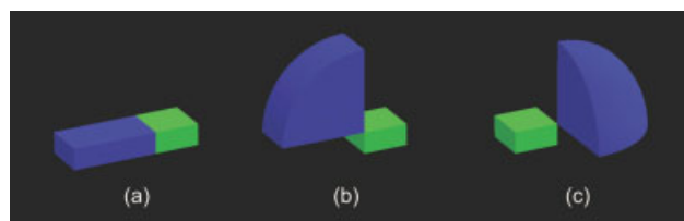
Figure 3. Interaction subregions. Sample interaction subregions are shown in blue, while the interaction box appears in green. One of the six face subregions is shown in (a), one of the 12 edge subregions in (b), and one of the eight corner subregions in (c).
