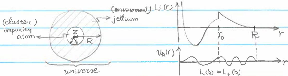
Method: Match a numerical wave function in the core to a plane wave outside.
