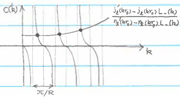
A rapid variation in  $[j'_L(kr_0) - j_L(kr_0)L_{-}(k)] / [n'_L(kr_0) - n_L(kr_0)L_{-}(k)]$  — resonance — gives rise to nonuniform distribution of the perturbed eigenenergies,  $k_n$ .
