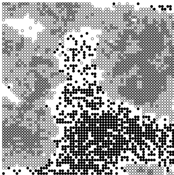
Fig. 7.5 Snapshot of part of a Pt-Ru electrode during a simulation of a linear sweep voltammetry experiment in which CO is replaced by OH. The Ru part of the electrode is completely covered by CO (gray circles) or OH (white circles). The Pt part is partially covered by CO (black circles) but a lot of it is vacant. The formation of OH on the electrode takes place initially on the Ru side of the Pt-Ru interface. That OH reacts with CO on the Pt side of the interface which leads to the vacancies on Pt. The vacancies on Ru are filled by new OH being formed [14]
